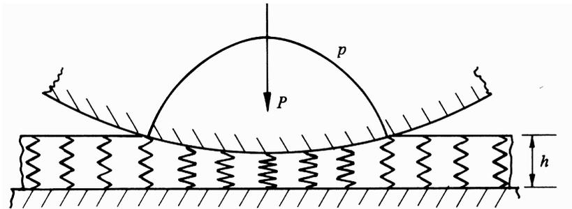
Fig. 1.2-3 Elastic foundation model (Johnson 1989)
