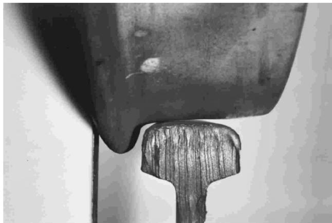
**Fig. 1.1-6** Wheel-rail contact (ISB, University of Hannover, Germany)
