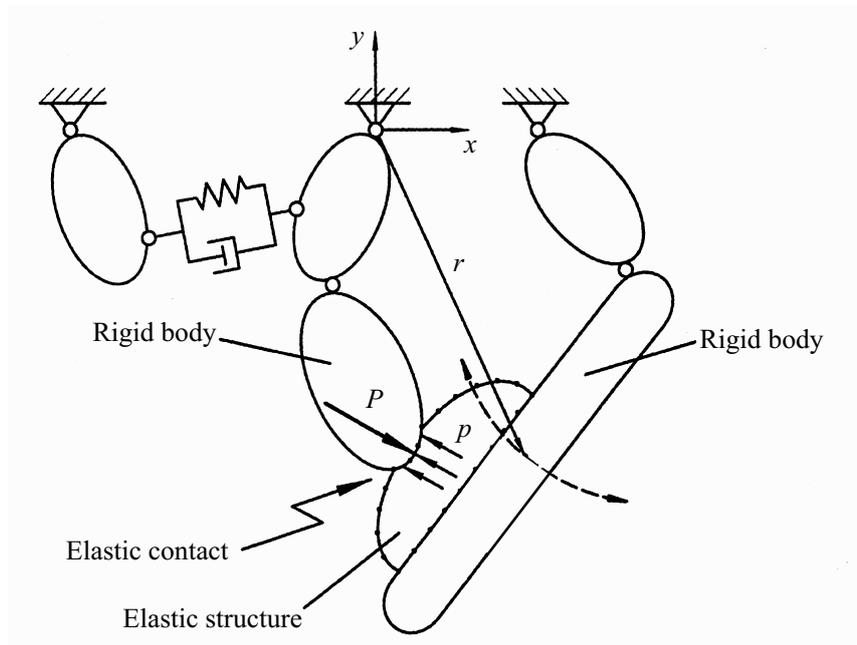
Fig. 1.2-2 Elastic Multibody System (ADAMS User Manual)
