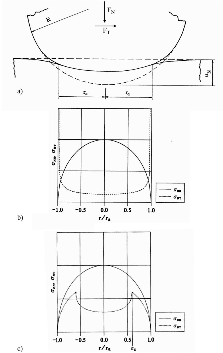
**Fig. 1.2-4** a) Hertzian normal contact of an elastic ball contacting an elastic half-space
