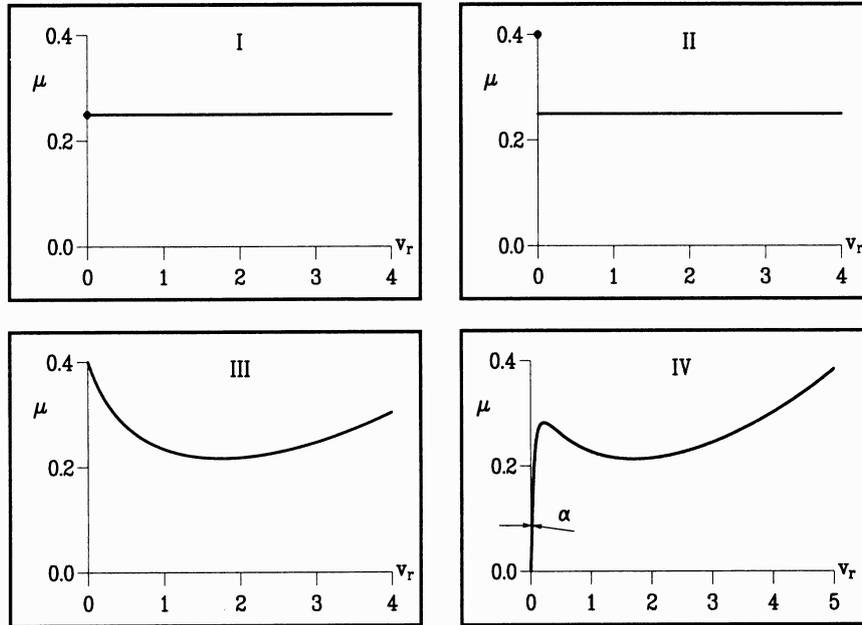
**Fig. 1.2-1** Friction coefficient characteristics (Hinrichs 1997a) **I**) Coulomb friction characteristic **II**) Coulomb-Amontons friction characteristic **III**) Identified friction characteristic **IV**) Smoothened friction characteristic
