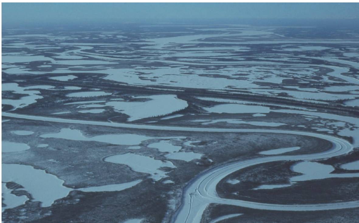
Fig. 1.2 The Mackenzie Delta in winter, showing an ice road built on a river channel (Photo C.R. Burn)
