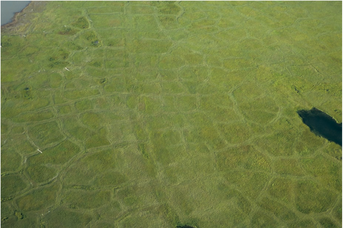
Fig. 1.4 Ice-wedge polygons in the outer Mackenzie Delta. The growth of ice wedges deforms the adjacent ground, raising the soil on either side of the wedge. The vegetation on
