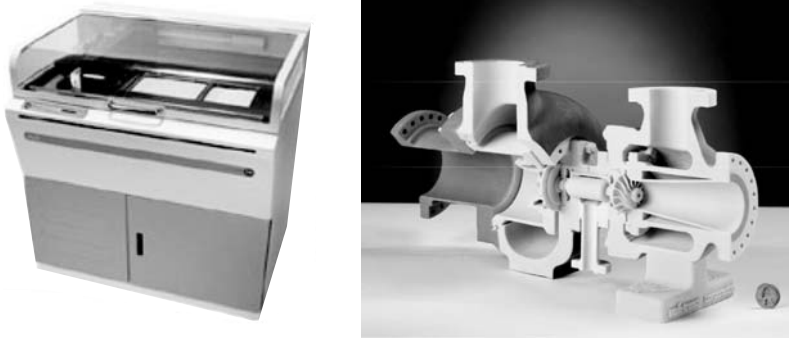
Figure 1.4 ZCorp Z406 machine along with some parts made using the colour capability (courtesy ZCorporation)
