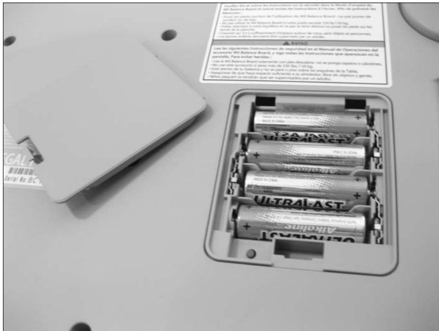
Figure 1-2: The Balance Board with the battery cover removed.
