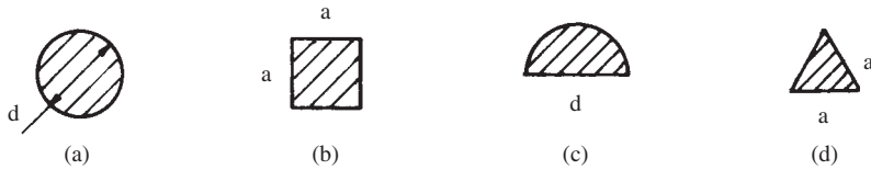
Figure 1.1 Standard, solid strut cross-sections
