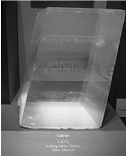
Figure 1.1 Double refraction in calcite. From http://www.physics.gatech.edu/gcuo/lectures .
