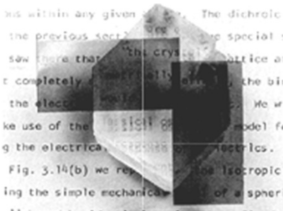
Figure 1.2 Two pieces of calcite at an angle. From http://www.physics.gatech.edu/gcuo/lectures .
