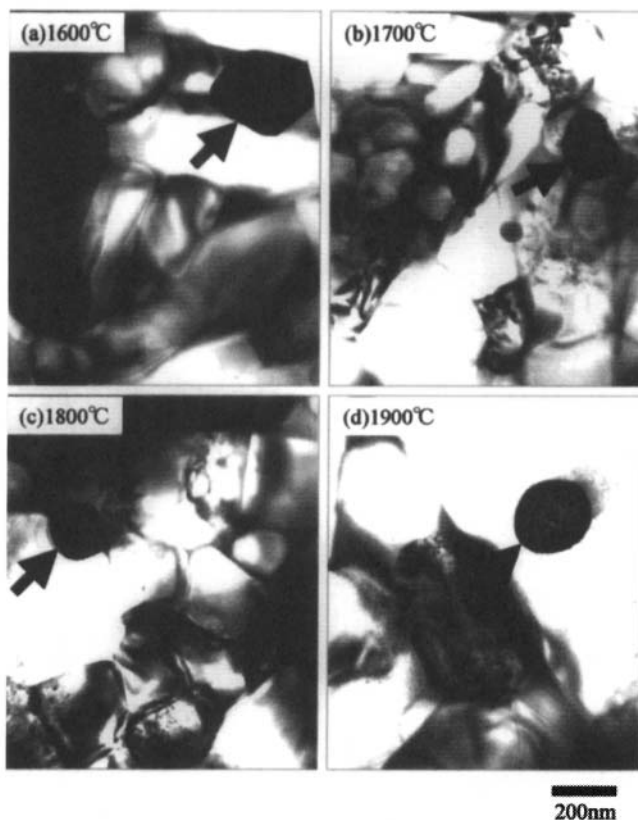
Fig. 6 TEM photographs of the 5wt%TiO 2 /5wt%AlN specimens fired at various temperatures for 1h in 0.9MPa N 2 . Arrow: TiN.
