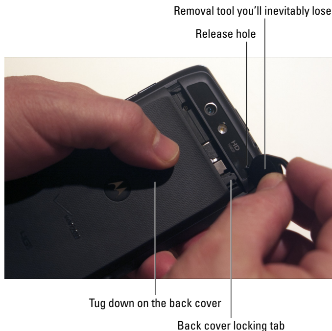
Figure 1-1: Removing the back cover.
