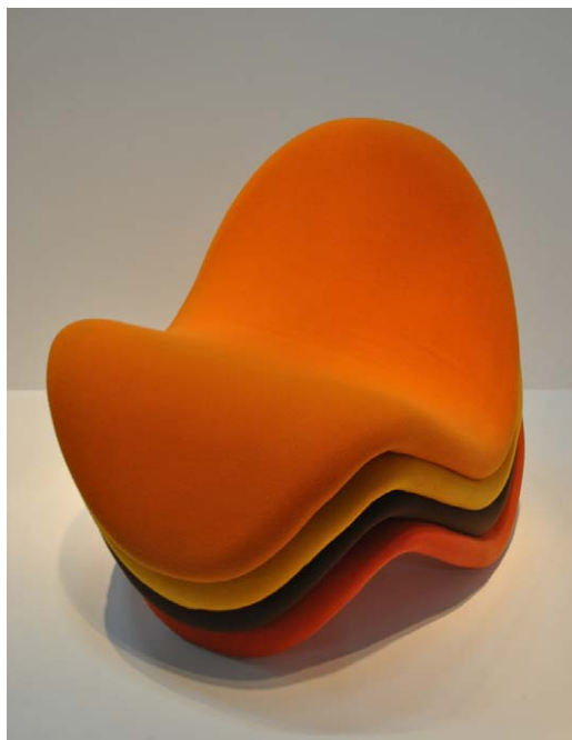
Figure P-3 Stacked Tongue 577 chairs, designed by Pierre Paulin (1967), tubular steel armature surrounded with rubber webbing and expanded foam, upholstered in polyester stretch fabric. Manufactured by Artifort. 33½ inches wide; 35½ inches deep; 24 inches high; 13¾ inches seat height (85 cm wide; 90 cm deep; 61 cm high; 34 cm seat height). Photography by Jim Postell, 2011.
