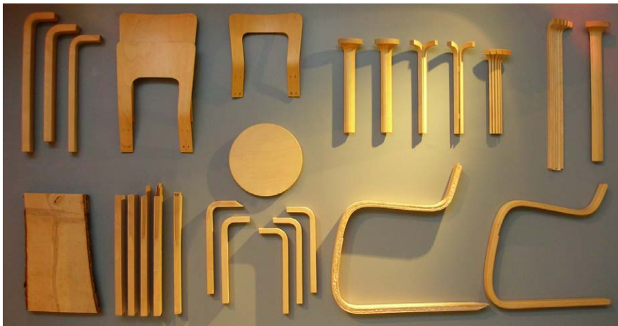
Figure P-1 Experiments with bent and laminated wood—furniture components for the Paimio Sanatorium and the library in Viipuri, Finland. Designed by Alvar Aalto. Photography by Jim Postell, 2006.
