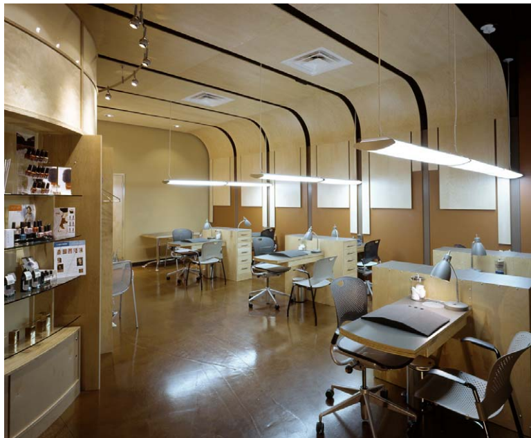
Figure 1.12 Built-in manicure stations at Alverno Salon and Spa, Cincinnati, Ohio. The storage units and manicure stations are mechanically attached to the floor and wall, enabling internal and continuous space for electrical power and air return ducts. Designed by Jim Postell, 2003. Photography copyright © Scott Hisey, 2004.
