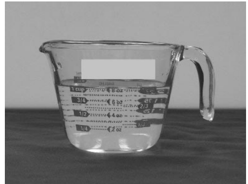
FIG. 1.2: Read the measure by holding it at eye level so the bottom of the meniscus matches the desired line on the side of the measure.
