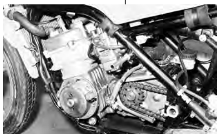
Final version of the HD 250, two-stroke featured monoshock rear suspension, just visible in the top right section of this photograph.
