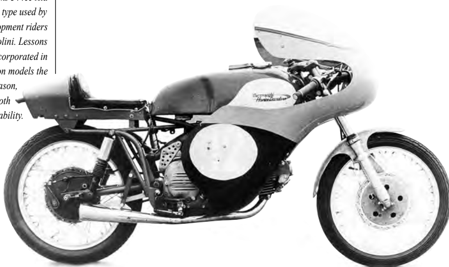
The Rickman brothers Don and Derek, built a batch of their Metisse frames for the Ala d'Oro engine, from an idea given to them by the Swiss rider/engineer, Othmar (Marly) Drixl. The first prototype appeared at the London Earls Court Show in late 1966.
