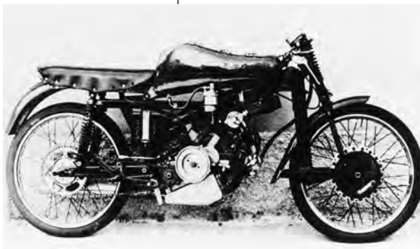
Little-known dohc single cylinder Aermacchi racing prototype, built in 1951 and intended as a challenge to the likes of FB Mondial and MV Agusta at Grand Prix level. It was never raced in a Grand Prix.
