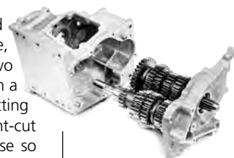
The 6-speed gearbox showing the housing cluster. Little known is that the factory also tested a 7-speed box. But FIM international regulations limited GP bikes to six, so the plan was dropped.
