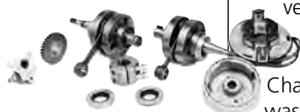
Crankshaft, ignition and rev counter drive details of the 250 Aermacchi twin. Note crank seals and cotter pin crankshaft coupling device. The ignition was manufactured by Dansi, who, like Aermacchi, were based in Varese.
