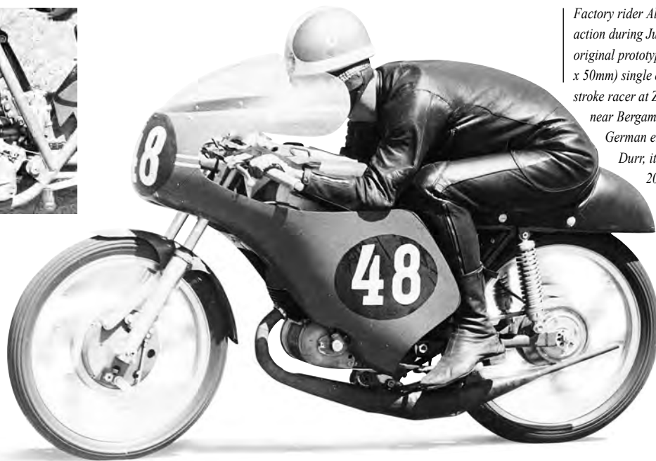
First seen at the 1969 Isle of Man TT this works 125 single raced by Kel Carruthers (and also Silvano Bertarelli) featured a twistgrip operated overdrive unit bolted on to the side of the original 5-speed gearbox. Like the earlier 50cc Kreidler, this effectively doubled up the available ratios, making ten in total.
