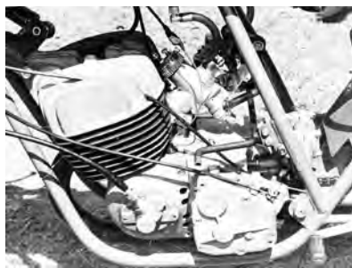
First seen at the 1969 Isle of Man TT this works 125 single raced by Kel Carruthers (and also Silvano Bertarelli) featured a twistgrip operated overdrive unit bolted on to the side of the original 5-speed gearbox. Like the earlier 50cc Kreidler, this effectively doubled up the available ratios, making ten in total.
