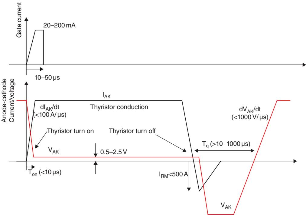
Figure 2.4 Thyristor switching characteristic.
