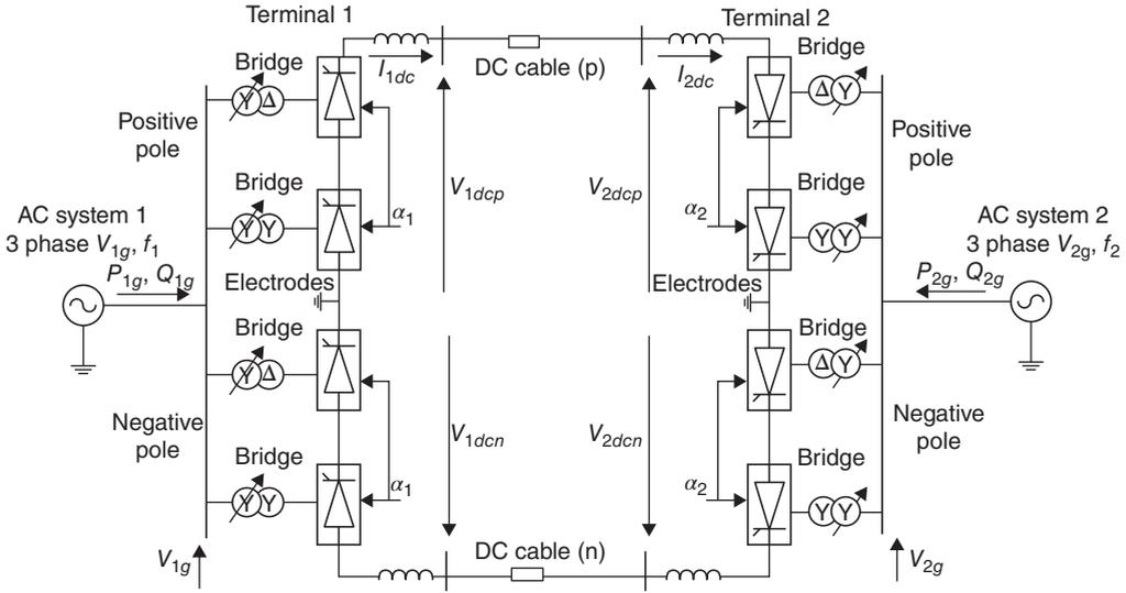
Figure 1.5 Bipolar HVDC (12-pulse) with ground return.
