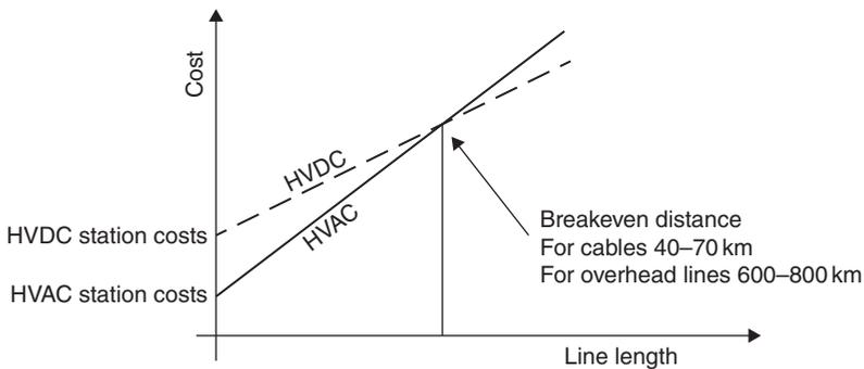
**Figure 1.1** HVDC and HVAC transmission cost comparison.
