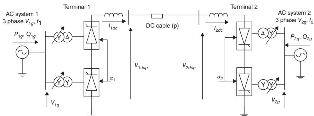
**Figure 1.4** Twelve-pulse monopolar HVDC with ground return.
