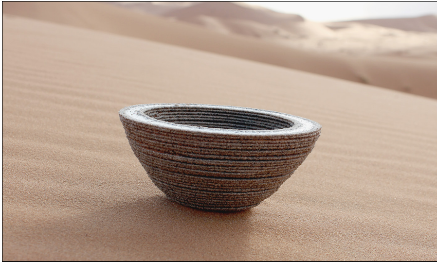
FIGURE 1-4: A glass bowl formed by passing sunlight through the Solar Sinter to fuse sand.
