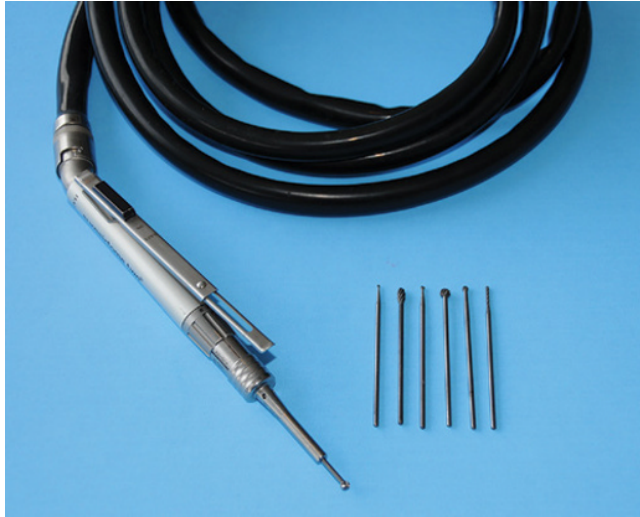
Figure 1.10 An electric (not shown) or pneumatic (illustrated) drill is used to gain access to the spinal canal. Burs of varying sizes are available and can be varied during the various stages of the drilling process.
