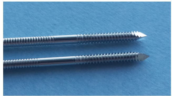
Figure 2.4 Imex Miniature Interface® pins (IMEX Veterinary Inc., Longview, TX, USA). These pins have a threaded tip and a roughened core to ensure a better grip of the acrylic cement. These are available in diameters from 0.9 to 2.4mm.
