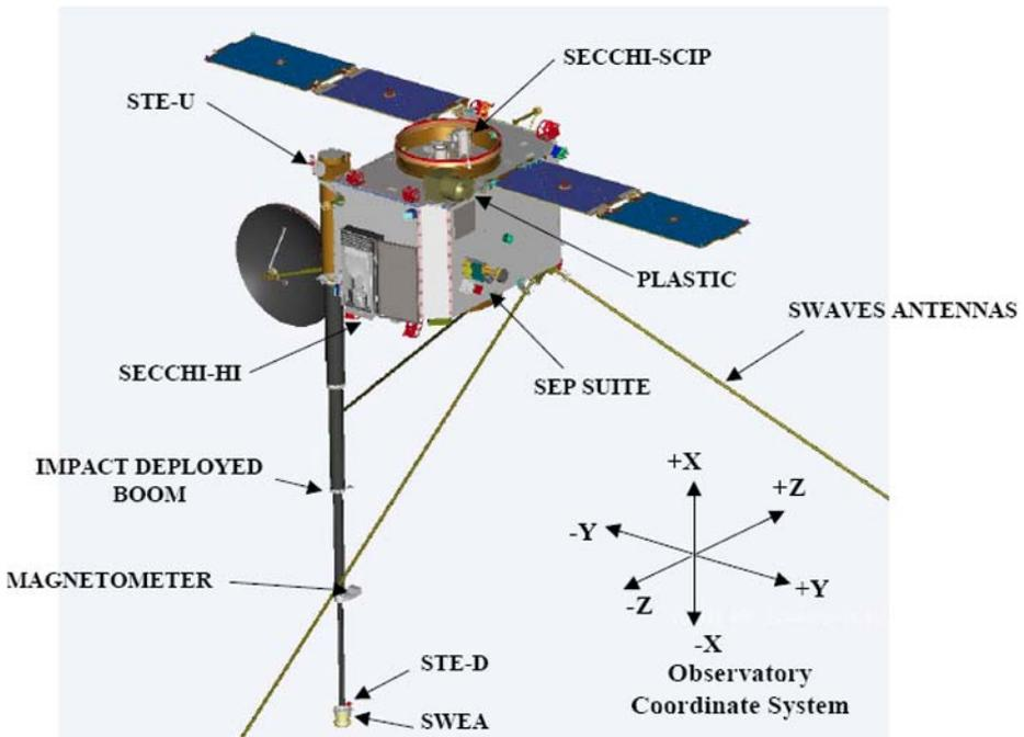
**Fig. 6** Illustration of spacecraft B in its deployed configuration. For scale, the large vertical boom (IMPACT boom) is approximately 6 m long
