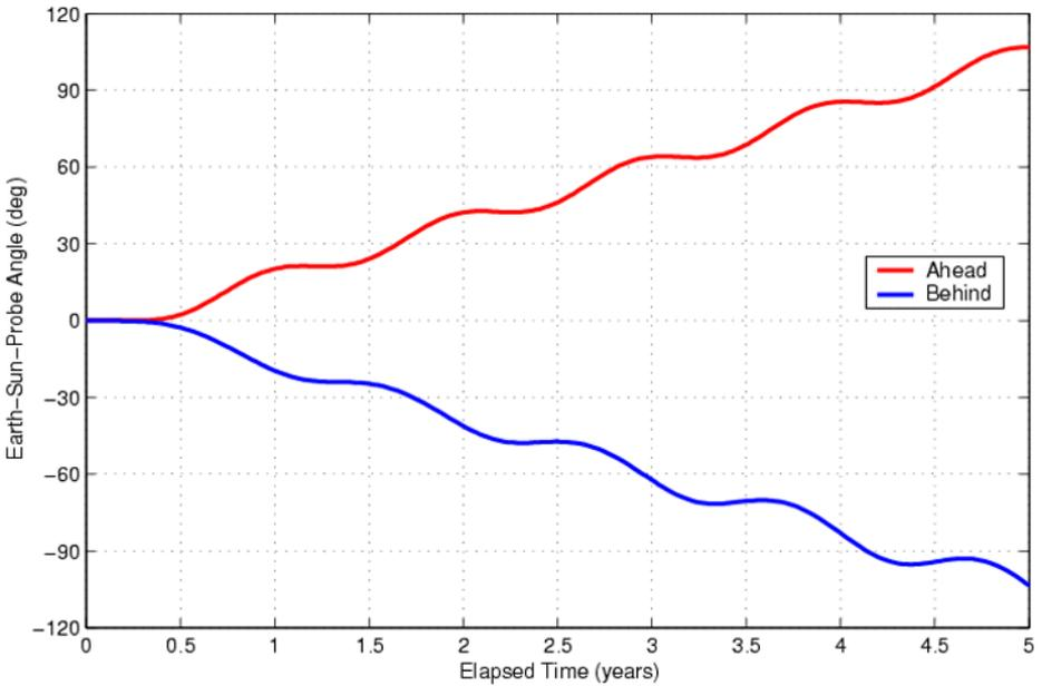
**Fig. 4** The graph shows the relative drift rates of the two observatories based on the prelaunch drift rates of 22° per year for observatory A and -22° per year for observatory B
