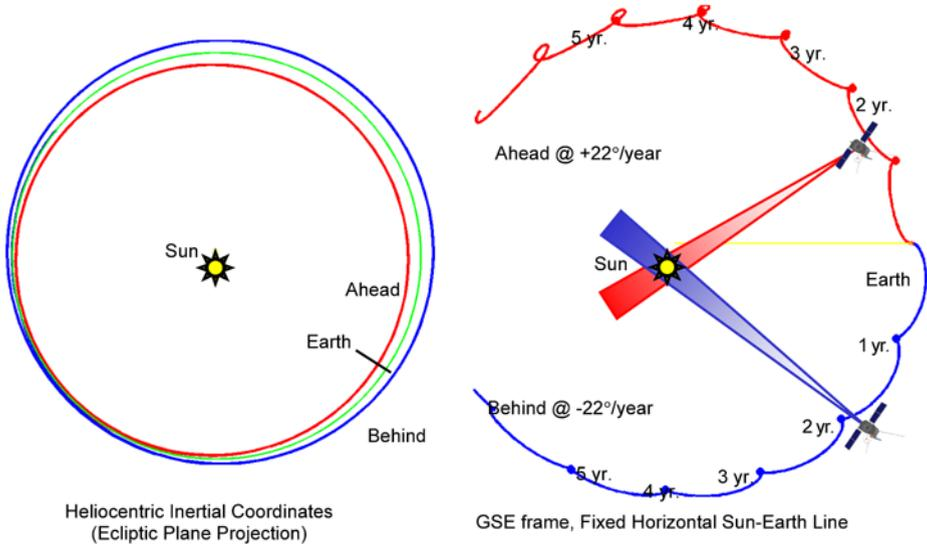
**Fig. 3** (a) The two observatory orbits projected onto the ecliptic plane. The projection shows the relative eccentricities of the orbits. (b) The same projection is shown but with a fixed Earth–Sun line. This figure shows the evolution of the relative geometries over the life of the mission
