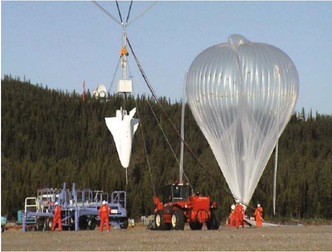
Frontispiece 7 High-speed flight demonstration through free fall from a balloon at high altitude. (courtesy of the National Aerospace Laboratory of Japan)
