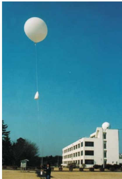
Frontispiece 8 Scene of the flight of a rawinsonde at the Aerological Observatory (Tsukuba, Japan). (Direction finding equipment has been installed in the dome on the roof of the government building, and this automatically tracks the rawinsonde and receives its signals)
