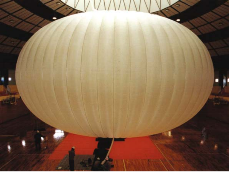
Frontispiece 5 Indoor inflation test of a super-pressure balloon based on a three-dimensional gore design
