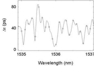
**Fig. 8.** DGD measurement of a fiber with mean DGD of 40 ps. The measured values of  $\Delta\tau$  appear reasonably constant over the bandwidth of the PSP, 0.025-nm. Markers indicate 0.1-nm intervals.
