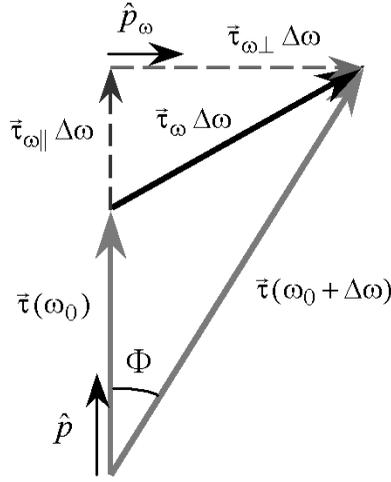
**Fig. 6.** Schematic diagram of the PMD vector  $\tau(\omega)$  and the second-order PMD components showing the change of  $\tau(\omega)$  with frequency. Note that  $\hat{p}_\omega$  is perpendicular to  $\hat{p}$ . The angular rotation rate,  $d\Phi/d\omega$ , of the PMD vector  $\tau(\omega)$  with  $\omega$  is described by  $|\hat{p}_\omega|$ .
