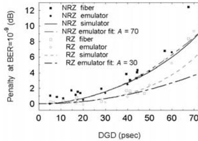
**Fig. 16.** NRZ and RZ penalties for measurements of real fiber and a first-order PMD emulator, as well as for simulations and optically preamplified receivers plotted as a function of instantaneous DGD. Worst-case polarization launch was used in all cases. Emulator fits use Eq. (31).
