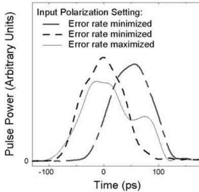
**Fig. 4.** Output pulse shapes for three polarization launches of a 10Gb/s, 50% duty cycle signal through a 48-km fiber with  $\sim 60$  ps PMD.
