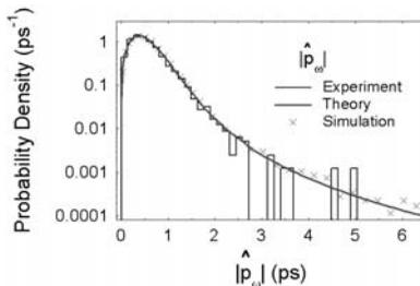
**Fig. 14.** Probability density for the depolarization of the principal states of polarization for a fiber with mean DGD of 1 ps.
