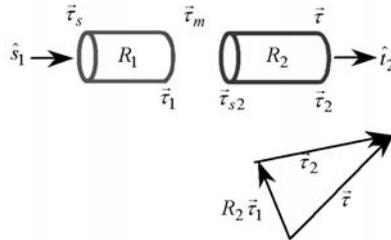
**Fig. 10.** Diagram of the concatenation of PMD vectors for two sections. The PMD vector  $\tau$  at the output is equal to the sum of  $\tau_1$  and  $\tau_2$ , after transforming by  $R_2$ .
