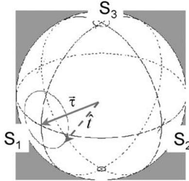
**Fig. 2.** Frequency-domain behavior of PMD in a short birefringent fiber, where the fiber's birefringent axis  $\tau$  is aligned with the  $S_1$  axis.
