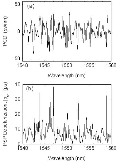
**Fig. 7.** (a) Plot of the polarization-dependent chromatic dispersion and (b) plot of PSP depolarization, for the same 14.7-ps mean DGD fiber as in Fig. 5.
