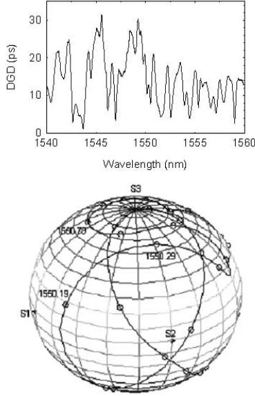
**Fig. 5.** PMD measurement of a 14.7ps mean DGD fiber. Top: Magnitude of  $\tau$ . Bottom: Direction of  $\tau$  (markers indicate 0.1-nm intervals).
