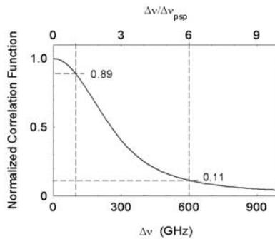
**Fig. 9.** Plot of the (normalized) correlation function,  $\langle \tau(\nu_0) \cdot \tau(\nu_0 + \Delta\nu) \rangle / \langle \Delta\tau^2 \rangle$ , as a function of the frequency separation,  $\Delta\nu$ , for a mean DGD of  $\overline{\Delta\tau} = 1.25$  ps and bandwidth of the PSP,  $\Delta\nu_{\text{PSP}} = 100$  GHz. The top  $x$  axis shows the normalized frequency separation,  $\Delta\nu/\Delta\nu_{\text{PSP}}$ , allowing general use of the plot.
