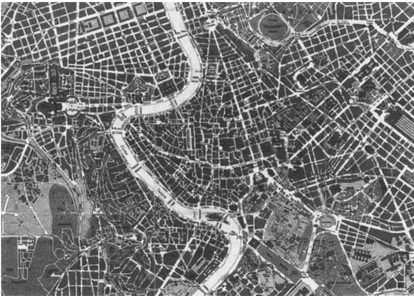
FIGURE 1.3. Plan of modern Rome, showing that in the ancient city (the center) the street length scales are considerably shorter than in the newer outskirts (Bejan 1997c)
