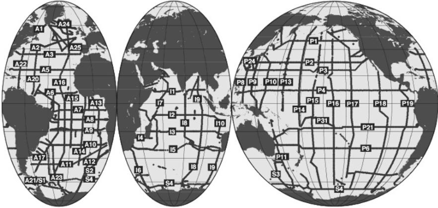
**Fig. 1.4.** Hydrographic sections for the WOCE Hydrographic Program one-time survey. Additional to these sections there are repeatedly surveyed hydrographic sections, XBT sections, current meter mooring arrays, satellite observations, surface drifters, subsurface floats, and tidal stations. Source: [http://woceatlas.tamu.edu/Sites/html/atlas/SOA\\_WOCE.html](http://woceatlas.tamu.edu/Sites/html/atlas/SOA_WOCE.html).
