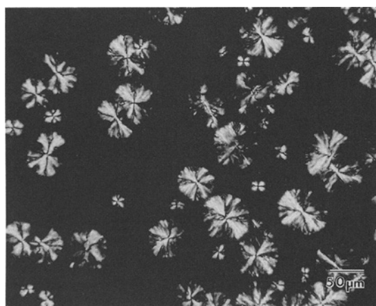
FIGURE 1.2. Polarized light micrograph of this polyoxymethylene film cooled from the melt shows recrystallization and formation of spherulites. The shape of the growing, birefringent spherulites is round.
