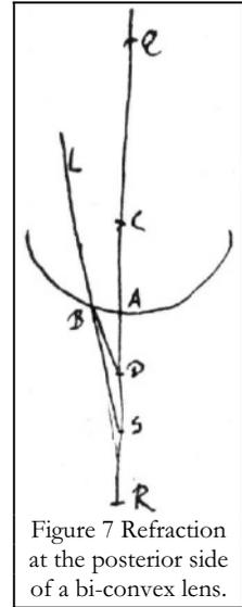
Figure 7 Refraction at the posterior side of a bi-convex lens.
