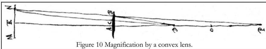
Figure 10 Magnification by a convex lens.
