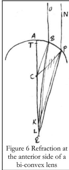
Figure 6 Refraction at the anterior side of a bi-convex lens
