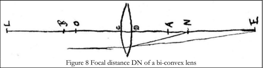
Figure 8 Focal distance DN of a bi-convex lens
