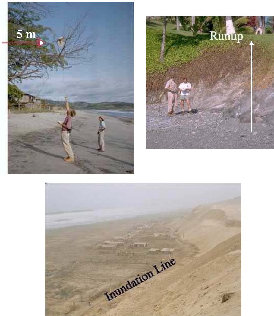
Fig. 2.: Photographs illustrating the definition and measurement of vertical flow depth (top left; 1992 Nicaragua tsunami), run-up (top right; 1995 Mexican tsunami), and inundation (bottom; 2001 Peru tsunami).
