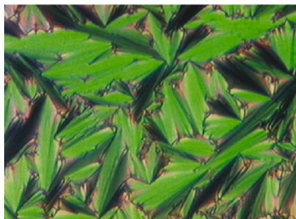
Figure 1-9. a) Schlieren texture of the SmAP A phase of compound 9a ; b) Fan-shaped texture of the SmAP A phase of compound 9a
