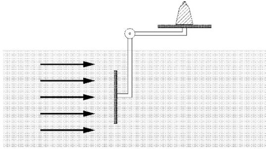
Fig. I-4. Force on a plate in a flow
