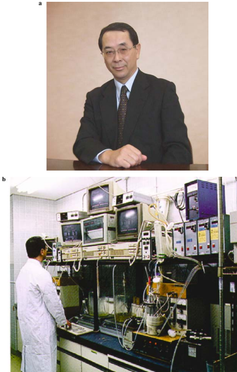
Fig. 1.1 (a) Dr. Hiroshi Kuriyama working with a continuous culture of Saccharomyces cerevisiae : (b) The continuous culture system. The impellers were driven by a 24 V motor (K; green line) and controlled by a power supply(A). Temperature was measured using a Pt 100 probe (yellow line) and controlled (B) to a user set-point by a 333 W heater (pink line). A water jacket (at 10°C) consisting of rubber tubing wrapped around the glass vessel (G) provides cooling (not shown). pH was measured using a steam sterilizable gel electrode connected (cyan line) to a (continued)
