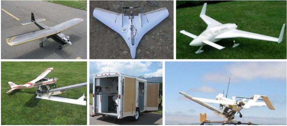
Fig. 1 The HUAS vehicle fleet includes (clockwise from top left) the CU Ares, the CU MUA, the Velocity XL, the MLB Bat 3, the CU ground control station, and the Hobico NextGen
