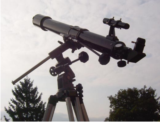
Fig. 1.2 A small refracting telescope on a low-cost mount. This telescope includes a small finder telescope, a right-angled prism, two low-cost eyepieces, a weight balance arm, and manual drives
