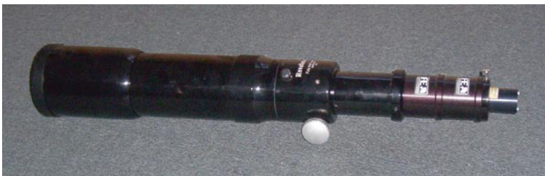
Fig. 1.5 An 80-mm refractor: ideal for wide-field views, when fitted to a suitable equatorial mount. Note the small CCD camera fitted to the eyepiece end of the telescope. In my case this is used for autoguiding (see later)
