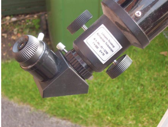
Fig. 1.3 The accessories that come with a small telescope usually include a right-angled prism. This enables the astronomer to view the heavens in a comfortable position rather than getting a cricked neck
