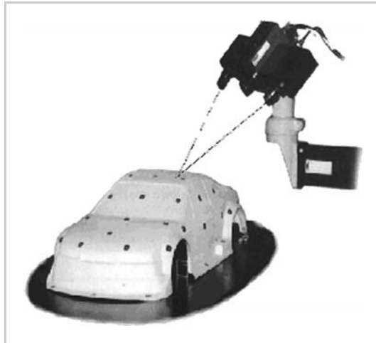
Figure 1.5. Optical scanning device. Originally published in Rapid Prototyping Casebook , McDonald, J.A., Ryal, C.J. and Wimpenny, D.I., 2001, © John Wiley and Sons Limited. Reproduced with permission.
