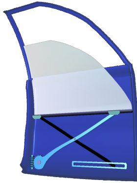
Fig. 3. An automobile power window
