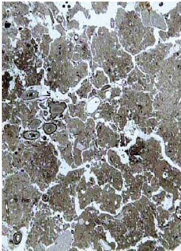
Fig. 4 Microphotograph of a vertically oriented soil thin section prepared from undisturbed samples from the surface layer (0–100 mm) of a loam soil (Lamelli-Calcaric Cambisol, according to FAO-IUSS-ISRIC classification, 1998) cropped with maize, showing an example of subangular blocky structure, where the aggregates are separated and surrounded by elongated continuous pores. The white areas represent the pores. Frame length 3 × 5 mm
