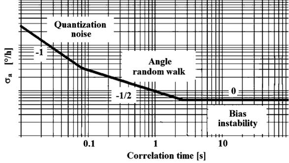
having slope equal to 0 is relevant to angle random walk. This means that the random walk noise is a white noise contribution to the angular velocity estimation. This can be explained observing that the rotation angle can be calculated by integrating the angular rate and, as previously explained, a random walk stochastic process is obtained by integrating a white noise stochastic process.
