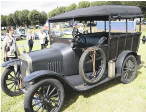
Fig. 1-8: The first series-production Ford T Model “Tin Lizzy” with rear wheel drive (standard layout) from 1908
