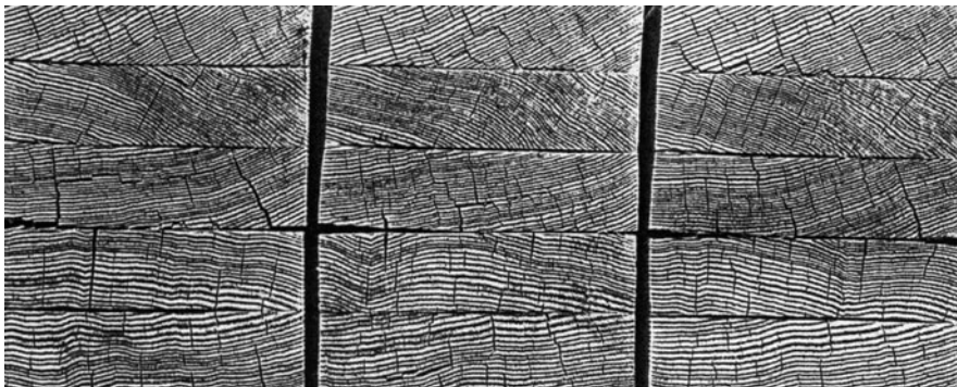
Fig. 1.1 Delamination observed on cross sections of Douglas-fir laminated lumber. Note delamination occurs predominantly in wood elements in the direction of medullary rays, frequently starting or finishing at the interface between the earlywood and latewood (Vick and Okkonen 2000, Figure 5a)
