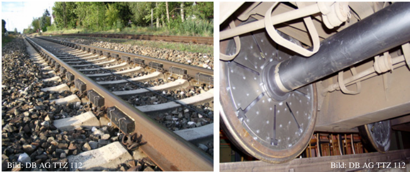
Fig. 2. DBs test track with rail dampers developed by Corus within the SILENCE project (left) and concept of the wheel dampers for freight wagons developed by Lucchini S.A. (right) (color figure online)
