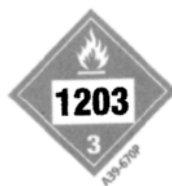
Figure 1.12 Gasoline Placard—Note the hazard class (three) shown in the lower point of the diamond.
