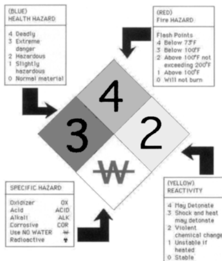
Figure 1.13 NFPA Label—This NFPA label outlines the four categories and shows what the numbers mean.
