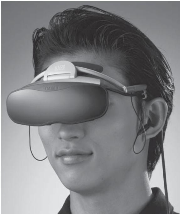
Figure 1.2 Head-mounted microdisplay GT270. Reprinted courtesy of Canon Inc.
