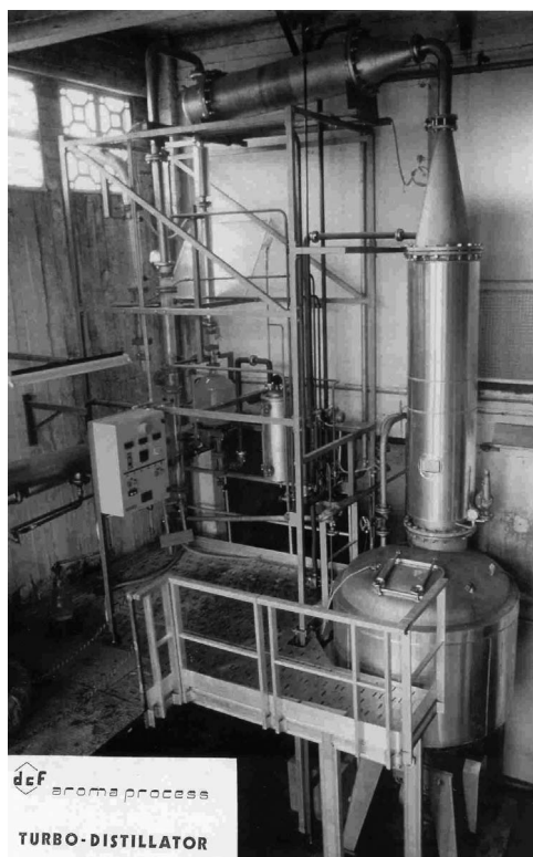
Figure 2.3. Turbodistillation of citrus essential oils.
