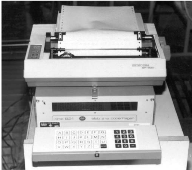
Figure 1.3 A data acquisition system for temperature measurements in cooling.
