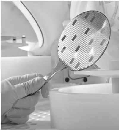
Figure 1.4 Silicon wafer, 100 mm in diameter, with about 200 device chips and a dozen test chips on it. Courtesy VTT
