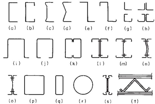
**Figure 1.2** Cold-formed sections used in structural framing.<sup>1,6</sup>
