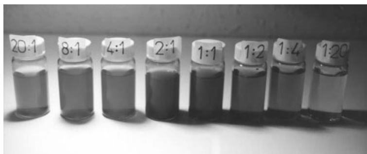
Figure 1.6 Photograph showing the solubility of complexes formed between Sudan red and polyvinylpyrrolidone in water at varying polymer:dye ratios. The dye is insoluble in water at polymer:dye ratios of <2:1 but is soluble at ratios of >4:1 .
