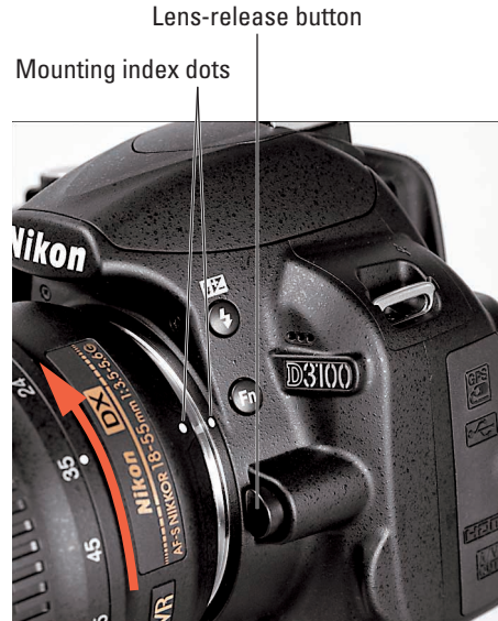
Figure 1-1: When attaching the lens, align the index markers as shown here.
