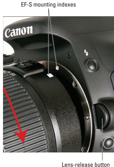
Figure 1-4: Place the lens in the lens mount with the mounting indexes aligned.
