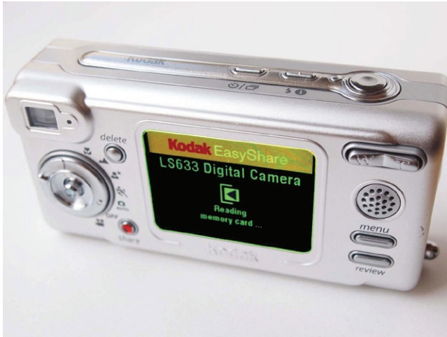
Figure 1.1 The first active-matrix OLED display product on the market (Kodak LS633 digital camera).
