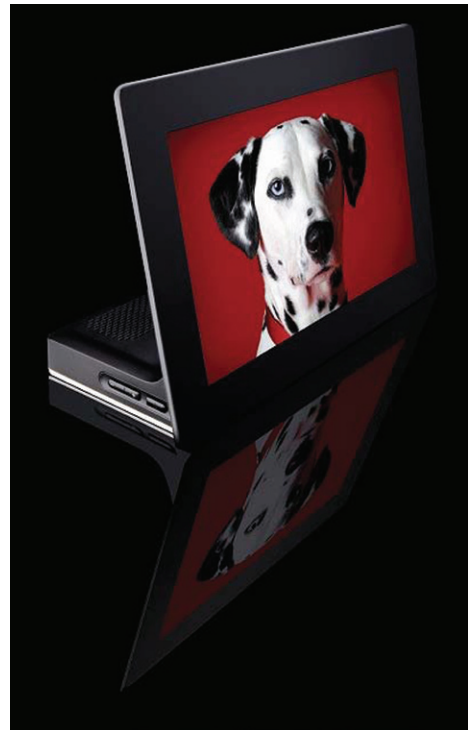
Figure 1.3 Example of a personal multimedia player using AMOLED (Dynaconnective Dawin; original equipment manufacturer [OEM] product of the Neosol Clid).
