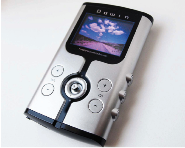
Figure 1.3 Example of a personal multimedia player using AMOLED (Dynaconnective Dawin; original equipment manufacturer [OEM] product of the Neosol Clid).
