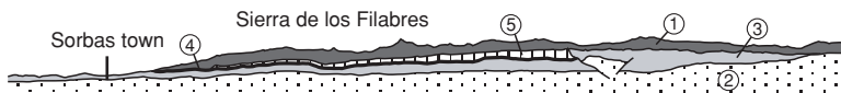
Fig. 2.2.4. Stop 4, Urra Mirador view to the north: 1, Nevado–Filabre basement of Sierra de los Filabres; 2, sandstones, siltstones and claystones from the Sorbas Member; 3, clays, silts, sands and limestones from the Zorreras Member; 4, marine bioclastic sandstones from the Lower Pliocene; and 5, Plio–Pleistocene Góchar Formation conglomerates. Vertical scale is exaggerated by 1.5.
