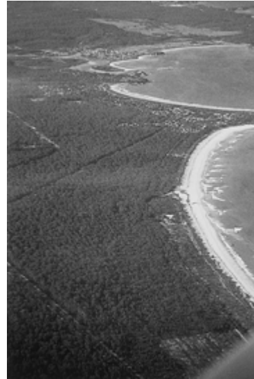
Fig. 1.8 Aerial photograph showing a strandplain coast where there is no significant estuary and no barrier island. Such a coast typically develops where there are no coastal bays and the gradient offshore is relatively steep, thus letting large waves reach the surf zone.
