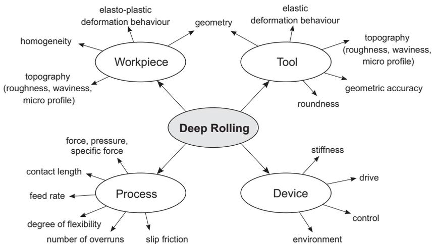
**Fig. 2.6:** Parameters influencing the results of deep rolling treatments
