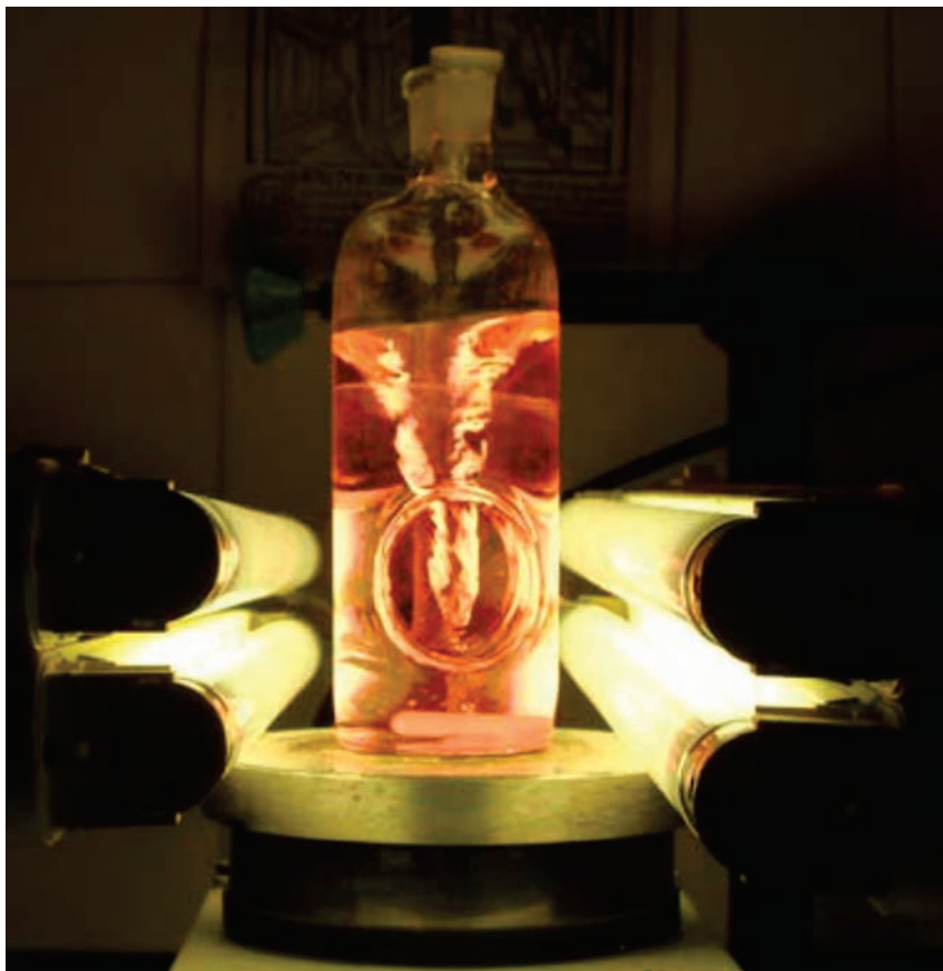
Figure 1.3 Two pairs of lamps used for external irradiation. In the arrangement shown, only a small fraction of the light flux is used.
