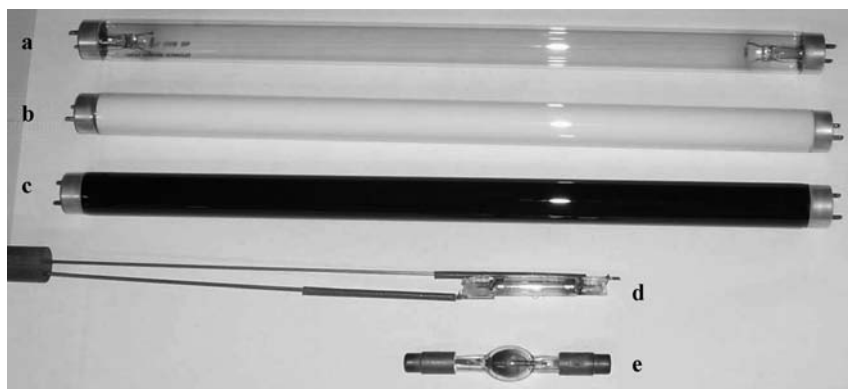
Figure 1.1 Lamps used for photochemical syntheses. (a) Low-pressure mercury arc; (b, c) phosphor-coated lamps, emission centered at 305 and 370 nm; (d, e) medium- and high-pressure mercury arcs, respectively.
