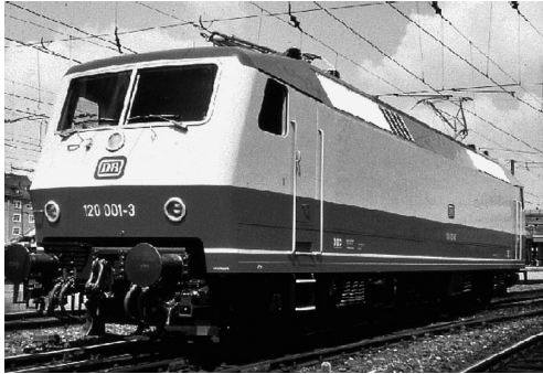
Fig. 1.9: Full-electric high-performance locomotive class 120 of DB; 1979, 5600 kW (Bombardier Transportation)
