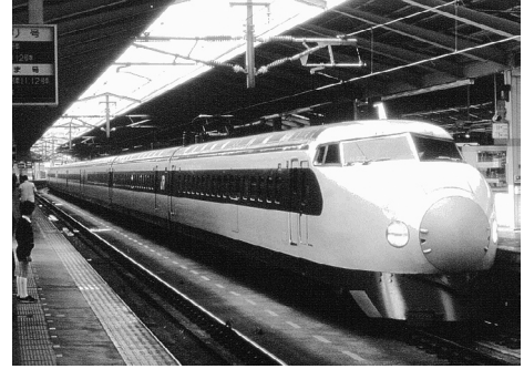
Fig. 1.6: Shin-Kansen High Speed Train of national railroad, Series 0; 220 kph
