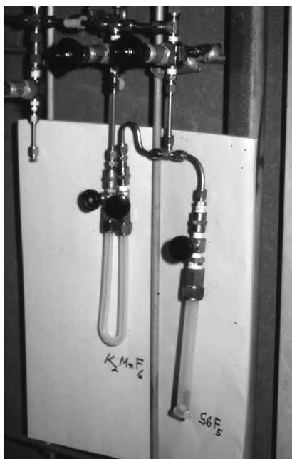
FIGURE 1.1 The original apparatus used by Christe in 1986 for the first chemical synthesis of F 2 . (For a color version of the figure, please see color plates.)
